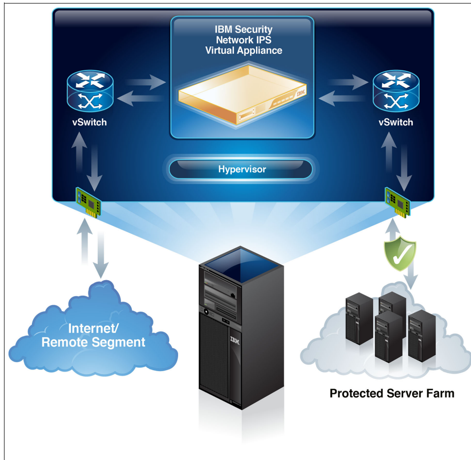
Figure 8-11 Virtual appliance on a physical server protecting a remote server farm
