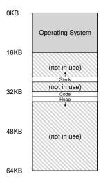
Figure 16.2: Placing Segments In Physical Memory
