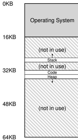
Figure 16.2: **Placing Segments In Physical Memory**
