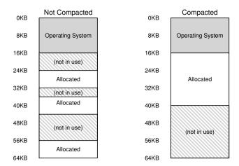
Figure 16.6: Non-compacted and Compacted Memory
