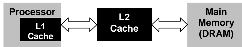
Figure 13-13 L1 and L2 Cache Placement
