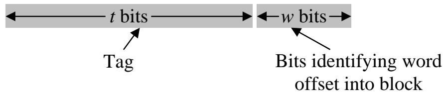
Figure 13-20 Fully Associative Partitioning of Memory Address
