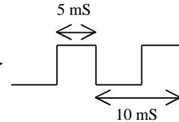
Duty cycle =  $(5\text{ms}/10\text{ms}) \times 100\% = 50\%$
