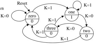
27. Create the next state truth table and the output truth table for the state diagram below. Use the variable names S<sub>1</sub> and S<sub>0</sub> to represent the most significant and least significant bits respectively of the binary number identifying the state. (8 points)
