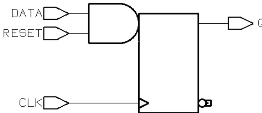
**D Flip-Flop With Synchronous and Asynchronous Load**
