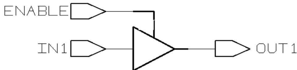
Example 6-66 provides an example of placing all high-impedance assignments in a single block. In this case, the data is gated and HDL Compiler infers a single three-state driver. Example 6-67 shows the inference report. Figure 6-24 shows the schematic the code generates.
