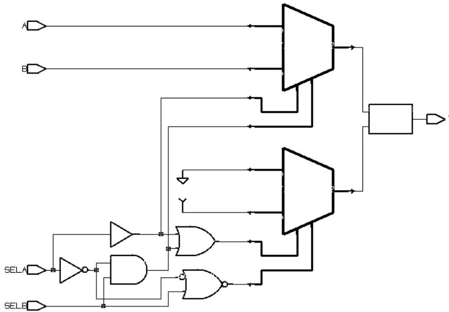
Example 6-68 provides an example of placing each high-impedance assignment in a separate block. In this case, HDL Compiler infers multiple three-state drivers. Example 6-69 shows the inference report. Figure 6-25 shows the schematic the code generates.
