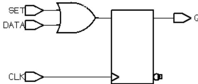
Example 6-35 provides the Verilog template for a D flip-flop with synchronous reset. HDL Compiler generates the verbose inference report shown in Example 6-36. Figure 6-14 shows the inferred flip-flop.
