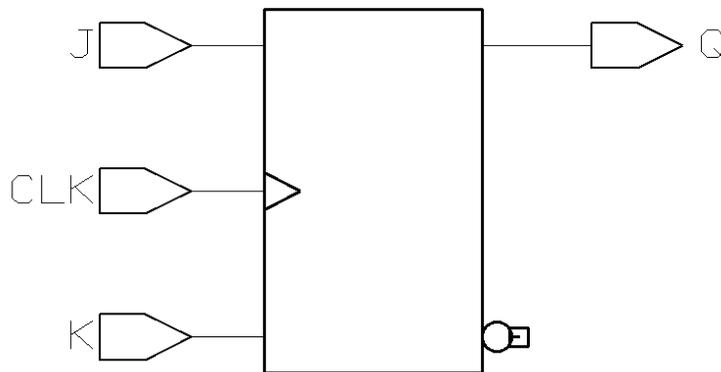
**JK Flip-Flop With Asynchronous Set and Reset**
