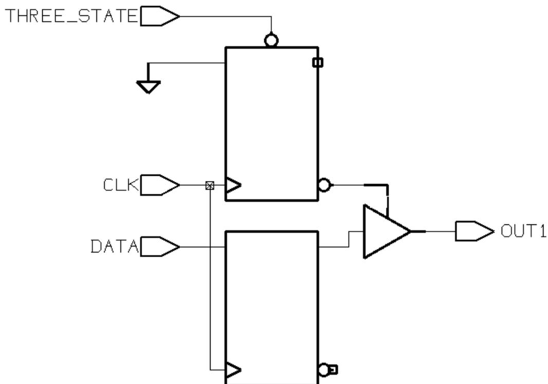
In Figure 6-26, the three-state gate has a register on its enable pin. Example 6-72 uses two blocks to instantiate a three-state gate, with a flip-flop only on the input. Example 6-73 shows the inference report. Figure 6-27 shows the schematic the code generates.
