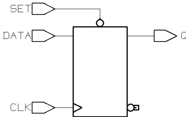
Example 6-29 provides the Verilog template for a D flip-flop with an asynchronous reset. HDL Compiler generates the verbose inference report shown in Example 6-30. Figure 6-11 shows the inferred flip-flop.
