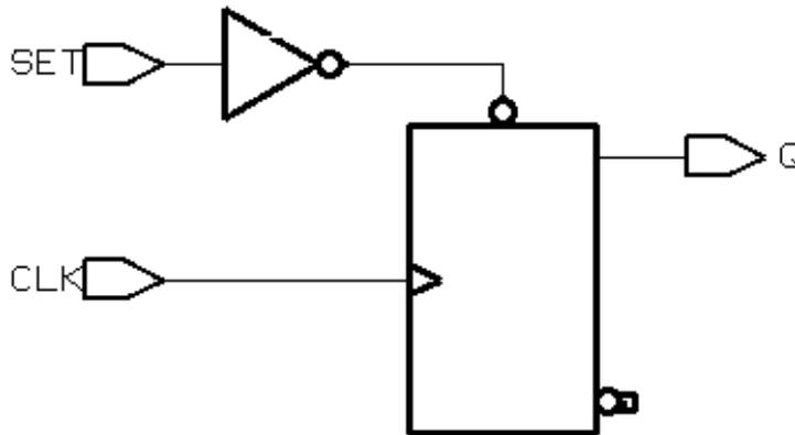
Example 6-47 provides the Verilog template for a toggle flip-flop with asynchronous reset. Example 6-48 shows the verbose inference report. Figure 6-20 shows the inferred flip-flop.
