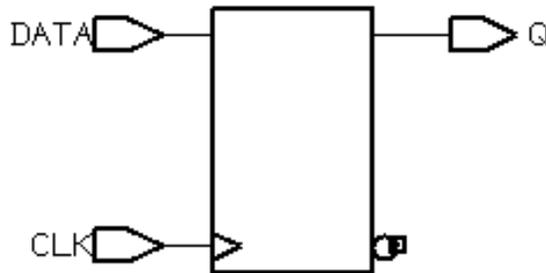
Example 6-25 provides the Verilog template for a negative-edge-triggered D flip-flop. HDL Compiler generates the verbose inference report shown in Example 6-26. Figure 6-9 shows the inferred flip-flop.
