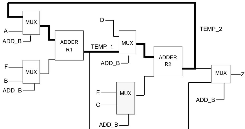
The circuit in Figure 7-1 is not faulty, because the multiplexing conditions never allow the entire path to be activated simultaneously. Still, the HDL Compiler resource sharing mechanism does not allow combinational feedback paths to be created, because most timing verifiers cannot handle them properly.
