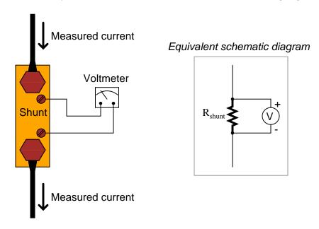
Suppose that a shunt resistance is labeled with the following rating: 150~A, 50~mV. What is the resistance of this shunt, in ohms? Express your answer in metric notation, scientific notation, and plain decimal notation.
