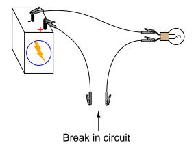
Try bridging this "break" with various materials, and note whether or not the light bulb lights up:
