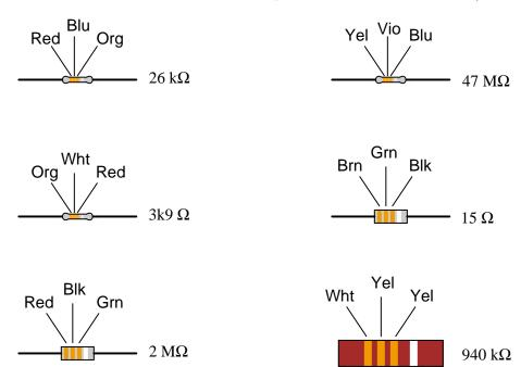
What patterns do you notice between the color codes (given as three-letter abbreviations, so as to avoid interpretational errors resulting from variations in print quality), the resistance values, and the physical sizes of the resistors?
