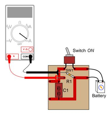
In order to measure current through resistor R1, one of its leads must be de-soldered from the circuit board so that the meter may be connected directly in-line (in *series*) with it.
