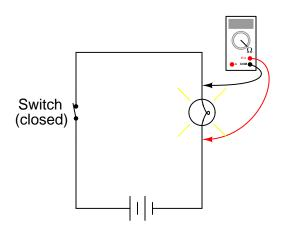
Suppose we needed to determine the resistance of the light bulb in this circuit, while energized:
