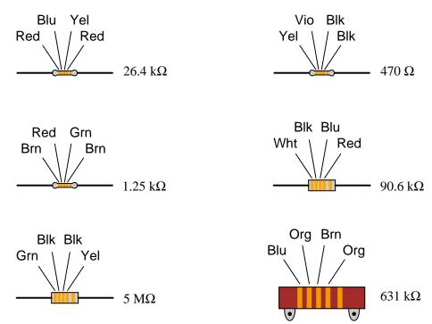
What patterns do you notice between the color codes (given as three-letter abbreviations, so as to avoid interpretational errors resulting from variations in print quality) and the resistance values of each resistor? Why do precision resistors use a "5-band" color code instead of a "4-band" color code?
