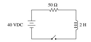
We may develop a loop equation based on Kirchhoff's Voltage Law, knowing that the voltage of the power source is constant (40 volts), and that the voltage drops across the inductor and resistor are  $V_L = L \frac{dI}{dt}$  and  $V_R = IR$ , respectively:
