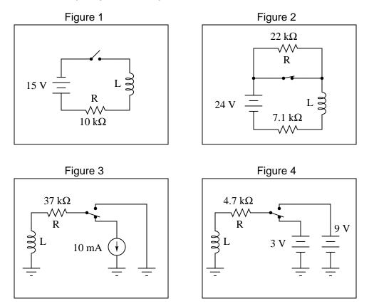
In each of these circuits, determine what the initial values will be for voltage across and current through both the inductor and (labeled) resistor. These will be the voltage and current values at the very first instant the switch changes state from where it is shown in the schematic. Also, determine what the final values will be for the same variables (after a large enough time has passed that the variables are all "settled" into their ultimate values).
