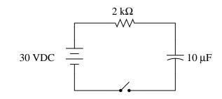
We may develop a loop equation based on Kirchhoff's Voltage Law, knowing that the voltage of the power source is constant (30 volts), and that the voltage drops across the capacitor and resistor are  $V_C = \frac{Q}{C}$  and  $V_R = IR$ , respectively:
