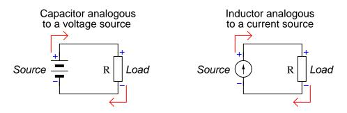
Large R values slow down RC circuits and speed up LR circuits, while small R values speed up RC circuits and slow down LR circuits.
