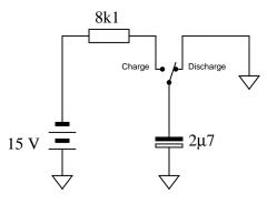
Suppose that the switch was left in the "discharge" position for some substantial amount of time. Then, someone moves the switch to the "charge" position to let the capacitor charge. Calculate the amount of capacitor voltage and capacitor current at exactly 45 milliseconds after moving the switch to the "charge" position.
