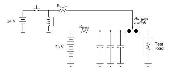
Suppose this surge power supply circuit failed to work after several months of good service. Nothing happens any more when the pushbutton switch is pressed and released. No spark is heard or seen in the air gap, and the test load receives no surge of current.
