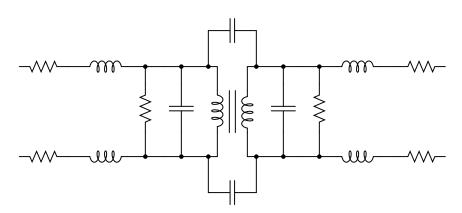
Each of these components is regarded as ideal (i.e., pure: possessing no parasitic characteristics), but together they "model" the behavior of a real transformer in terms readily applicable to existing mathematical techniques.
