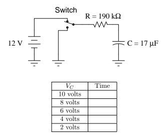
Trace the direction of electron flow in the circuit, and also mark all voltage polarities.  $\underline{file~02943}$
