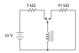
Now, assume that the switch is *instantly* moved to the right-hand position. How much voltage will the inductor initially drop?
