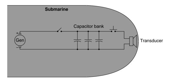
As you might well imagine, such a capacitor bank can be lethal, as the voltages involved are quite high and the surge current capacity is enormous. Even when the DC generator is disconnected (using the "toggle" disconnect switch shown in the schematic), the capacitors may hold their lethal charge for many days.
