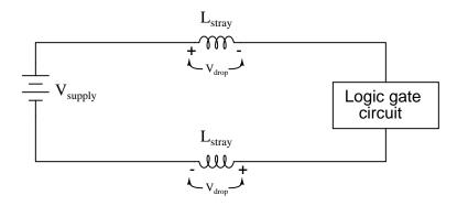
Suppose a logic gate circuit creates transient currents of 175 amps per nanosecond (175 A/ns) when switching from the "off" state to the "on" state. If the total inductance of the power supply conductors is 10 picohenrys (9.5 pH), and the power supply voltage is 5 volts DC, how much voltage remains at the power terminals of the logic gate during one of these "surges"?
