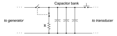
Suppose the capacitor bank consists of forty 1500  $\mu$ F capacitors connected in parallel (I know the schematic only shows three, but . . .), and the discharge resistor is 10 k $\Omega$  in size. Calculate the amount of time it takes for the capacitor bank to discharge to 10 percent of its original voltage and the amount of time it takes to discharge to 1 percent of its original voltage once the disconnect switch opens and the discharge switch closes.
