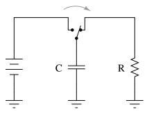
Would a larger capacitance value result in a slower discharge, or a faster discharge? How about a larger resistance value? You may find the "Ohm's Law" equation for capacitance helpful in answering both these questions:
