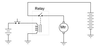
The problem here is every time the pushbutton switch is released, the contacts arc significantly. This happens because the inductor releases all of its stored energy as a high-voltage spark across the opening contacts. *Inductive kickback* is the phrase commonly used to describe this effect, and over time it will prematurely destroy the switch.
