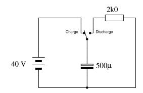
Suppose that the switch was left in the "charge" position for some substantial amount of time. Then, someone moves the switch to the "discharge" position to let the capacitor discharge. Calculate the amount of capacitor voltage and capacitor current at exactly 3 seconds after moving the switch to the "discharge" position.
