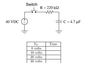
Trace the direction of electron flow in the circuit, and also mark all voltage polarities.  $\underline{file~02942}$
