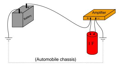
What is the purpose of having a capacitor connected in parallel with the amplifier's power terminals? What benefit does this give to the audio system, overall?
