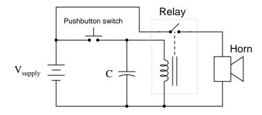
To calculate the amount of time the horn will remain on after the pushbutton switch is released, we must know a few things about the relay itself. Since the relay coil acts as a resistive load to the capacitor, we must know the coil's resistance in ohms. We must also know the voltage at which the relay "drops out" (i.e. the point at which there is too little voltage across the coil to maintain a strong enough magnetic field to hold the relay contacts closed).
