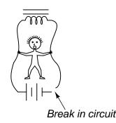
At the time, I didn't understand how inductance worked. I only understood how to make magnetism with electricity, but I didn't realize a coil of wire could generate (high voltage!) electricity from its own magnetic field. I did know, however, that the 9 volts output by the battery was much too weak to shock me (yes, I touched the battery terminals directly to verify this fact), so *something* in the circuit must have generated a voltage greater than 9 volts.
