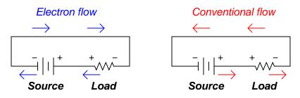
Whichever notation you choose to follow in your analysis of circuits, the understanding should be the same: the reason voltage polarities across the resistor and battery differ despite the same direction of current through both is the flow of power. The battery acts as a *source*, while the resistor acts as a *load*.
