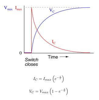
$V_C = \underline{1.9915 \text{ volts}} @ t = 3 \text{ seconds}$
