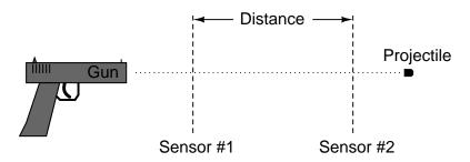
A crude intervalometer may be constructed using two thin wires as sensors, which are broken by the passage of the projectile. The two wires are connected in an RC circuit as such:
