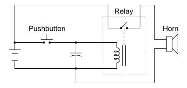
Suppose this circuit has functioned as designed for quite some time, then one day develops a problem. The horn sounds immediately when the pushbutton is pressed (as it should), bit it immediately silences instead of continuing to sound for a few more moments when the pushbutton is released. Based on this information, identify these things:
