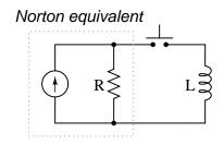
Re-analyze the circuit in this form, and try to explain why more resistance makes the inductor charging time faster and less resistance makes the inductor charging time slower. <u>file 03533</u>
