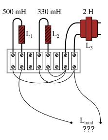
Also, write a formula that calculates total inductance given the values of inductors  $L_1$ ,  $L_2$ , and  $L_3$ . file 00379
