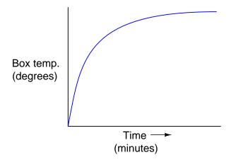
An engineer approaches you and says she wants you to build an electrical circuit that *models* this thermal system. What kind of circuit would you consider building for the engineer, to make a realistic electrical analogue of the box's temperature? Be as specific as you can in your answer.  $\frac{file \ 01218}{file \ 01218}$
