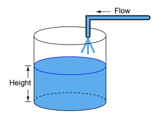
In calculus terms, we would say that the tank *integrates* water flow into water height. That is, one quantity (flow) dictates the rate-of-change over time of another quantity (height).
