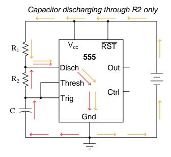
Note that this second current (through the battery) does not go anywhere near the capacitor, and so is irrelevant to the discharge cycle time.
