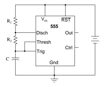
In this configuration, the "555" chip acts as an *oscillator*: switching back and forth between "high" (full voltage) and "low" (no voltage) output states. The time duration of one of these states is set by the charging action of the capacitor, through both resistors ( $R_1$  and  $R_2$  in series). The other state's time duration is set by the capacitor discharging through one resistor ( $R_2$ ):
