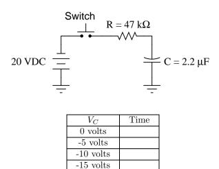
Trace the direction of current in the circuit while the capacitor is charging, and be sure to denote whether you are using electron or conventional flow notation.
