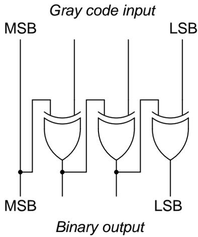
Challenge question: this circuit is not as suited to high-speed conversion as a binary-to-Gray converter, even though it uses the same quantity and same type of logic gate. Explain why problems may arise if this circuit is forced to convert Gray code inputs that are changing rapidly (for instance, translating the output of a Gray-code rotary encoder into binary, when the mechanical encoder is rotating at a very high speed).
