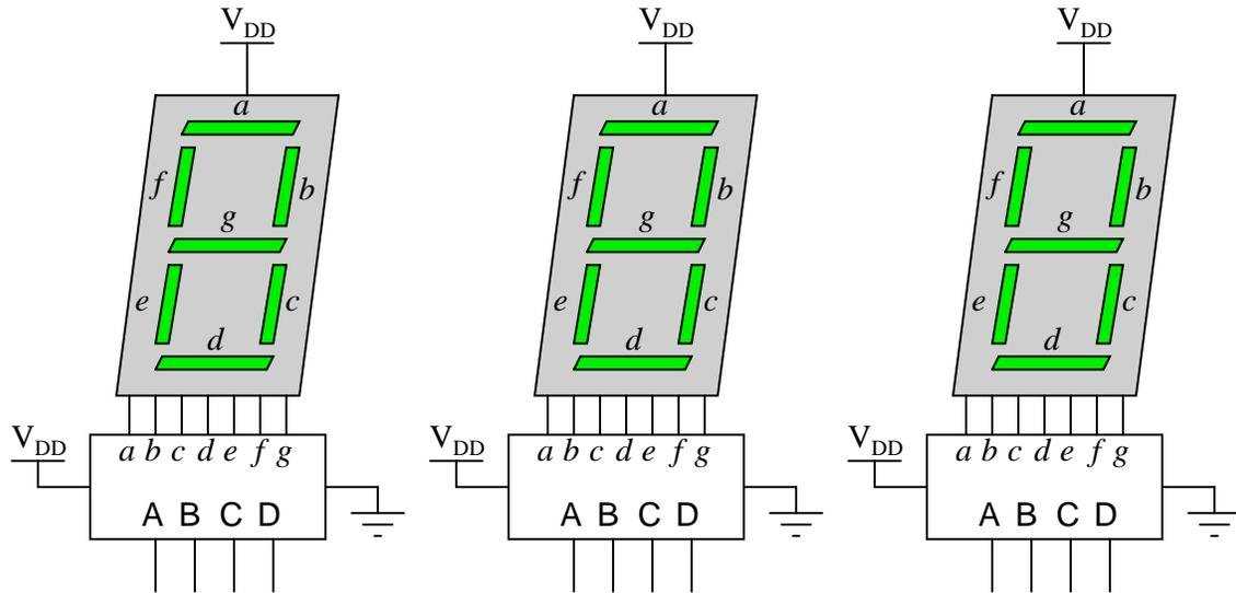
If we are driving the decoder ICs with a microprocessor or microcontroller, this direct technique unfortunately uses a lot of I/O pins. In this particular case, with three 7-segment displays, we would need to use *twelve* output pins on the microcontroller for the three BCD numbers:
