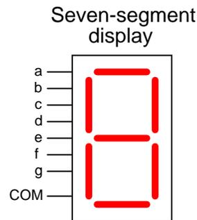
A special decoder circuit is needed to translate 4-bit BCD codes into the particular combinations of segment activations that represent decimal digits.
