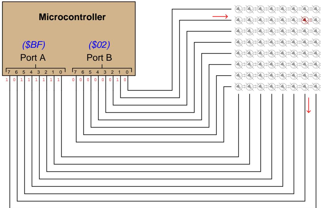
Note that a *high* state is required on one of port B's pins to activate a row, and a *low* state is required on one of port A's pins to activate a column, because the LED anodes connect to port A and the LED cathodes connect to port B.
