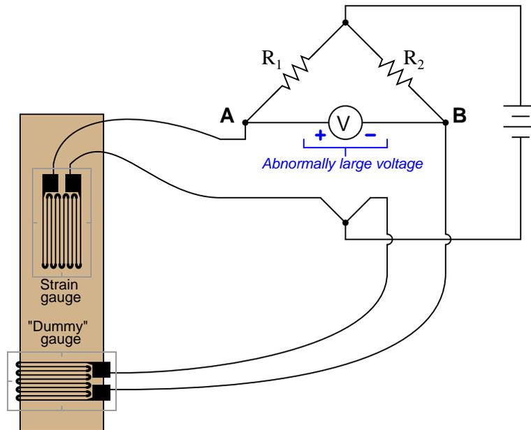
Something is wrong in the bridge circuit, because this voltage is present even when there is no physical stress on the specimen. Identify which of the following faults could cause the excessive voltage to appear across the voltmeter, and which could not. Consider only one of these faults at a time (no multiple, simultaneous faults):
