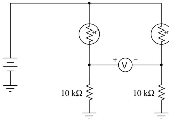
The  $+t^\circ$  label in each one shows that they both have positive  $\alpha$  coefficients.
