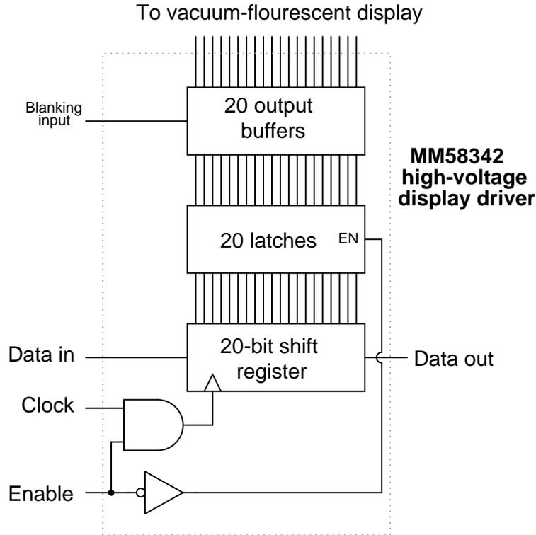
Read the datasheet for this device, then comment on why you think a serial (rather than parallel) data input format was chosen. Also describe the sequence of operation for loading data into this IC and outputting that data to the 20 output lines.
