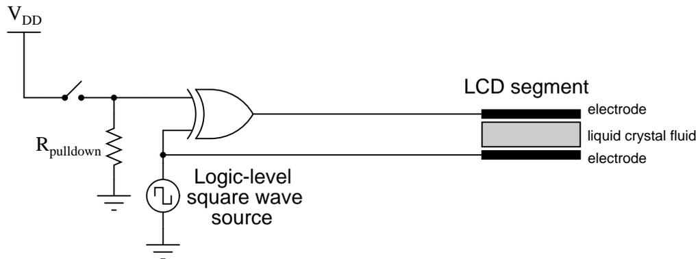
Consider the square wave voltage source in this schematic as a source of alternating "high" and "low" logic states, 5 volts and 0 volts respectively. Determine what sort of voltage exists across the liquid crystal fluid with the switch in the open position as well as the closed position, and from this determine which switch position results in a *darkened* LCD versus a *transparent* LCD.
