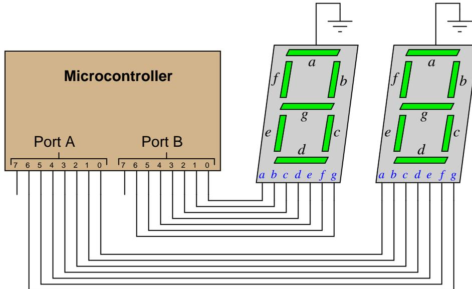
Write the necessary hexadecimal values to be output at ports A and B to generate the display "42" at the two 7-segment display units.
