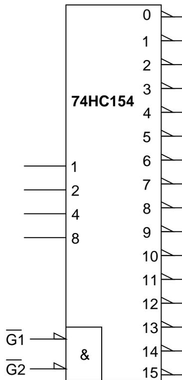
What terminal(s) do we use for the signal input, if using this chip as a *demultiplexer* and not just a decoder?
