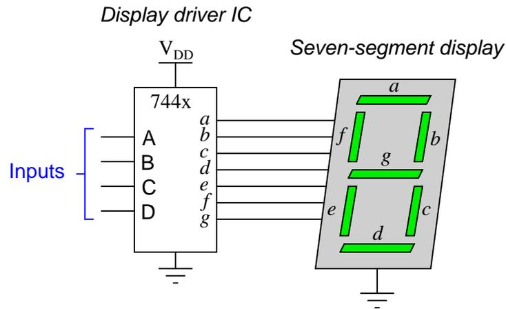
The student using the 7448 notices the LED segments glowing faintly, but the patterns are not correct for the digits that are supposed to be displayed. The student using the 7447 has an even worse problem: no light at all! Both have checked and re-checked their wiring, to no avail. It seems as though all the connections are in the right place.
