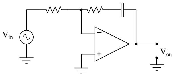
What type of filtering function (low pass, high pass, band pass, band stop) is provided by both these filter circuits? Comparing these two circuit designs, which one do you think is more practical? Explain your answer.
