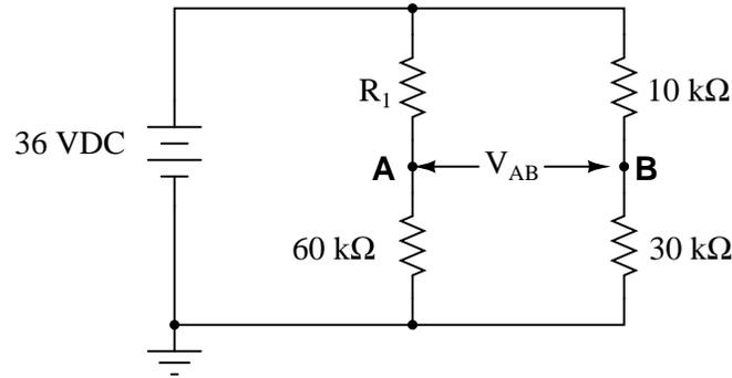
How much resistance must  $R_1$  possess in order to drop that amount of voltage?
