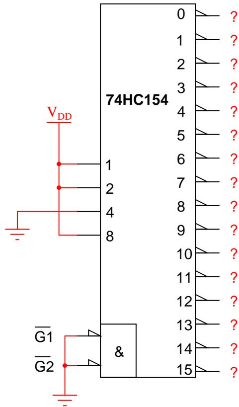
Identify the logic states of all output terminals given the input conditions shown.
