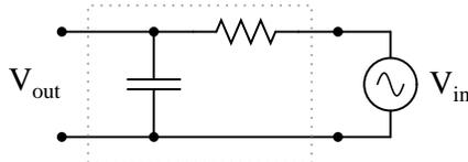
Calculate the impedance of both the resistor and the capacitor at this frequency. What do you notice about these two impedance values?
