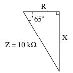
We know that the *sine* function relates the sides X and Z of this impedance triangle with the 65 degree angle, because the sine of an angle is the ratio of *opposite* to *hypotenuse*, with X being opposite the 65 degree angle. Therefore, we know we can set up the following equation relating these quantities together:
