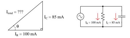
Calculate the total current and the angle  $\Theta$  of the total current, explaining your trigonometric method(s) of solution.
