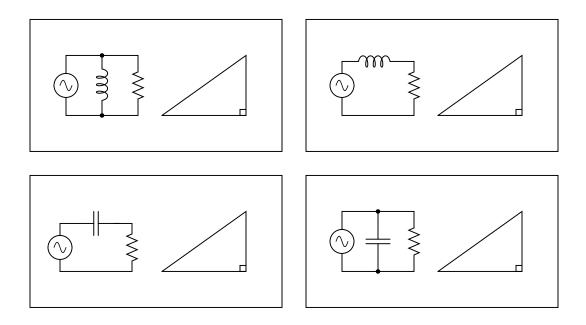
Use a triangle to calculate the total voltage of the source for this series RC circuit, given the voltage drop across each component:
