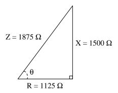
Since all side lengths on this triangle are known, there is no need to apply the Pythagorean Theorem. However, we may still calculate the two non-perpendicular angles in this triangle using "inverse" trigonometric functions, which are sometimes called *arc*functions.
