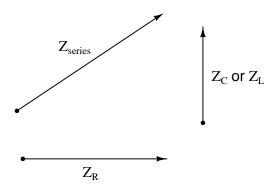
Since the phasor for resistive impedance  $(Z_R)$  has an angle of zero degrees and the phasor for reactive impedance  $(Z_C \text{ or } Z_L)$  either has an angle of +90 or -90 degrees, the *phasor sum* representing total series impedance will form the hypotenuse of a right triangle when the first to phasors are added (tip-to-tail).
