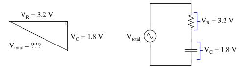
Explain what equation(s) you use to calculate  $V_{total}$ , as well as why we must geometrically add these voltages together.
