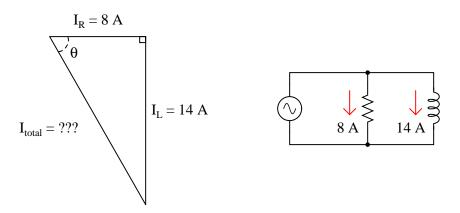
Calculate the total current and the angle  $\Theta$  of the total current, explaining your trigonometric method(s) of solution.
