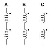
If one end of each winding pair were connected together at a common ground point, and each winding pair output 70 volts RMS, how much voltage would be measured between any two open wires?
