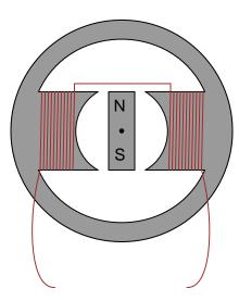
(The actual magnet polarities are not essential to the answer. Without knowing which way the coils were wound and which way the rotor is spinning, it is impossible to specify an exact magnetic polarity, so if your answer had "N" facing down and "S" facing up, it's still acceptable.)
