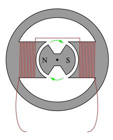
Hint: how many cycles of AC are produced for every revolution of the rotor?  $\underline{\text{file }00819}$
