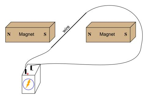
Is this an example of an electric motor or an electric generator?  $\underline{{\rm file}~00382}$
