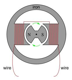
What factors determine the magnitude of this voltage? According to Faraday's Law, what factors can we alter to increase the voltage output by this generator?
