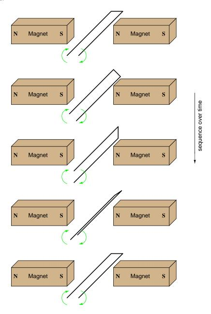
Describe the nature of the voltage induced in the stationary ("stator") windings, as the permanent magnet rotor rotates in this machine:
