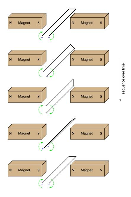
Challenge question: if a resistor were connected between the ends of this wire loop, would it "see" direct current (DC), or alternating current (AC)?
