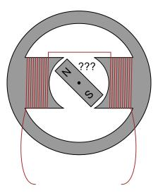
If this alternator is spun at 4500 RPM (revolutions per minute), what will be the frequency of its output voltage?
