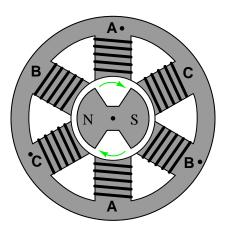
Each pair of windings in each set is series-connected, so they act as just three separate windings (pay close attention to the phase-marking dots!):
