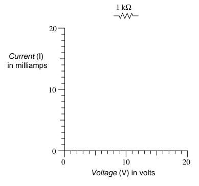
Plot this graph, following Ohm's Law. Then, plot another graph representing the voltage/current relationship of a 2 k $\Omega$  resistor.
