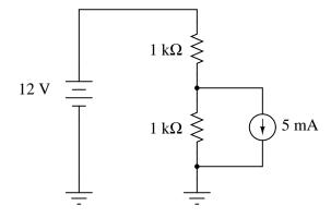
Hint: it may help you to set up the necessary equation by labeling the current through the lower resistor as I and the current through the upper resistor as I + 0.005.
