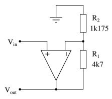
Algebraically manipulate the gain equation to solve for  $R_2$ , then determine the necessary value of  $R_2$  in this circuit to give it a voltage gain of 6.8.
