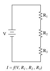
"I is some function of V,  $R_1$ ,  $R_2$ , and  $R_3$ "
