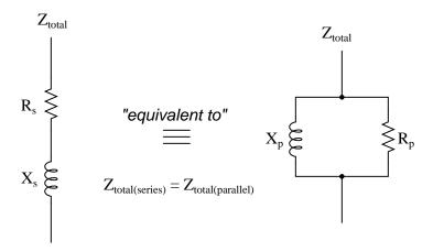
Series and parallel LR networks, if truly equivalent, should share the same Q factor as well as sharing the same impedance. Develop an equation that solves for the Q factor of a parallel LR circuit.
