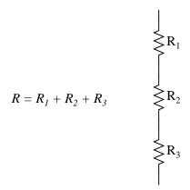
Combine these two equations together using substitution so that we have a single equation for calculating current I in a three-resistor series circuit given the source voltage V and each resistance value  $R_1$ ,  $R_2$ , and  $R_3$ :
