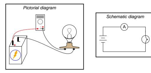
In order to practically function, an ammeter must have some internal resistance. It is usually a very small amount, but it does exist. It should be apparent to you that the presence of this resistance will have some effect on the circuit current, when compared to the amount of current in the circuit without any meter connected:
