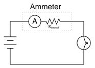
Explain why it is usually safe to ignore the internal resistance of an ammeter, though, when it is in a circuit. A common term used in electrical engineering to describe this intentional oversight is *swamping*. In this particular circuit an engineer would say, "The resistance of the light bulb *swamps* the internal resistance of the ammeter."
