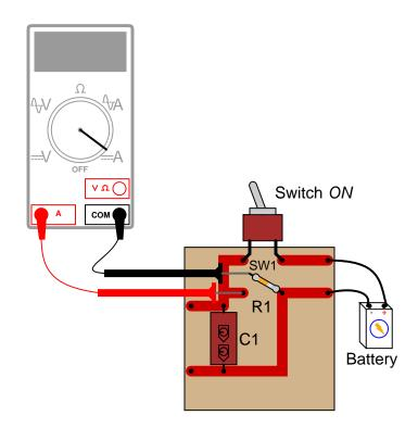
In order to measure current through resistor R1, one of its leads must be de-soldered from the circuit board so that the meter may be connected directly in-line (in *series*) with it.
