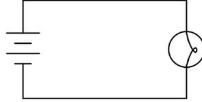
Other orientations of the components within the diagram are permissible. What matters, though, is for there to be a single, continuous path for electric current from the battery, to the light bulb, and back to the other terminal of the battery.
