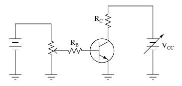
Procedure: measure the voltage dropped across  $R_C$  while varying  $V_{CC}$ , for several different values of  $I_B$  (inferred by measuring voltage drop across  $R_B$ ).
