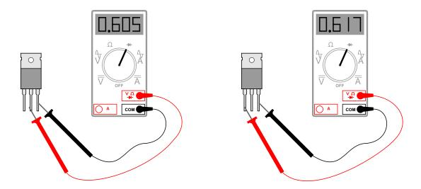
From these measurements, determine what type of BJT this is (PNP or NPN) and identify all three terminals.
