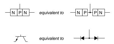
Acting on this idea, the student proceeds to connect two 1N4001 rectifying diodes back-to-back and try to use it as a transistor. This idea does not work: although the diode pair reads the same patterns of continuity as a transistor would, it does not amplify. Explain why.
