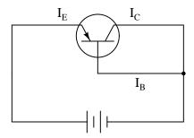
Which current is the smallest and which is the largest? Are there any two currents that are closer in magnitude than with the third? If so, which currents are they?
