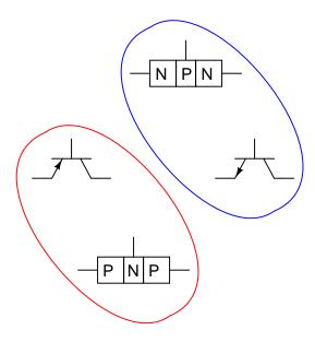
Follow-up question: identify the terminals on each transistor schematic symbol (base, emitter, and collector).
