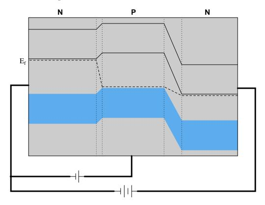
Trace the paths of injection, diffusion, and collection currents in this energy diagram for a PNP transistor as it is conducting:
