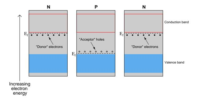
The presence of dopants in the semiconducting materials creates differences in the Fermi energy level  $(E_f)$  within each piece.
