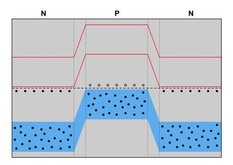
"Injection" current consists of those majority charge carriers (either electrons or holes, depending on the transistor type) that are "injected" from the emitter region into the base region of a transistor. "Diffusion" current is the current through the base terminal of the transistor resulting from recombination of electrons and holes in the emitter-base junction. Most of the injection current, however, becomes "collection" current and goes through the collector terminal of the transistor.
