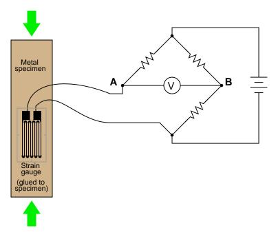
Explain what would happen to the voltage measured across this bridge circuit  $(V_{AB})$  if the strain gauge were to be *compressed*, assuming that the bridge begins in a balanced condition with no strain on the gauge. file 00547
