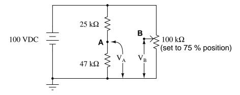
Now, calculate the voltage between points  ${\bf A}$  (red lead) and  ${\bf B}$  (black lead). file 00542
