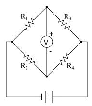
Also, write an equation containing only the four resistor values  $(R_1, R_2, R_3, \text{ and } R_4)$  showing their relationship to one another in a balanced condition.
