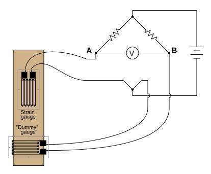
The following bridge circuit uses two strain gauges (one to measure strain, the other to compensate for temperature changes), the amount of strain indicated by the voltmeter in the center of the bridge. Unfortunately, though, it has a problem. Instead of registering a very small voltage as it normally does, the voltmeter shows a large voltage difference, with point  $\bf A$  positive and point  $\bf B$  negative:
