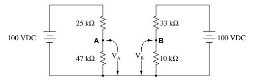
Now, calculate the voltage between points  ${\bf A}$  (red lead) and  ${\bf B}$  (black lead) ( $V_{AB}$ ). file 01725
