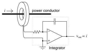
Connected as such, the output of the integrator circuit will be a direct representation of the amount of current going through the wire.
