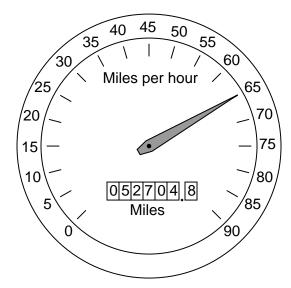
On this one instrument, two measurements are given: speed in miles per hour, and distance traveled in miles. In areas where metric units are used, the units would be kilometers per hour and kilometers, respectively. Regardless of units, the two variables of speed and distance are related to each other over time by the calculus operations of integration and differentiation. My question for you is which operation goes which way?
