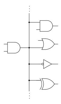
Explain why this limit exists. What is it about the construction of CMOS logic gates that inherently limits the number of CMOS inputs that any one CMOS output can drive? What might happen if this limit is exceeded?
