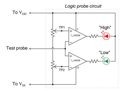
When this logic probe circuit is connected to the  $V_{DD}$  and  $V_{SS}$  power supply terminals of a powered CMOS circuit, what voltage levels should test points TP1 and TP2 be adjusted to, in order for the probe to properly indicate "high" and "low" CMOS logic states? Consult a datasheet for the quad NAND gate numbered 4011. This is a legacy CMOS integrated circuit. file 01275
