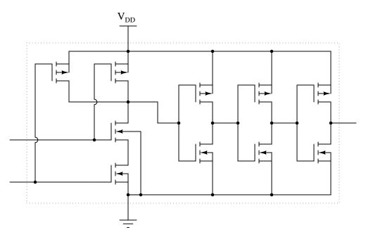
As far as the basic logic function is concerned, the additional transistors are unnecessary. However, the "buffering" they provide does serve a useful function. What is that function? Are there any disadvantages to buffered logic gates, versus unbuffered?
