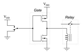
Normally, it would be considered good design practice to connect a commutating diode in parallel with the relay coil, to prevent high-voltage transients when the coil is de-energized. However, this is not necessary when a CMOS gate drives a coil. Explain why.
