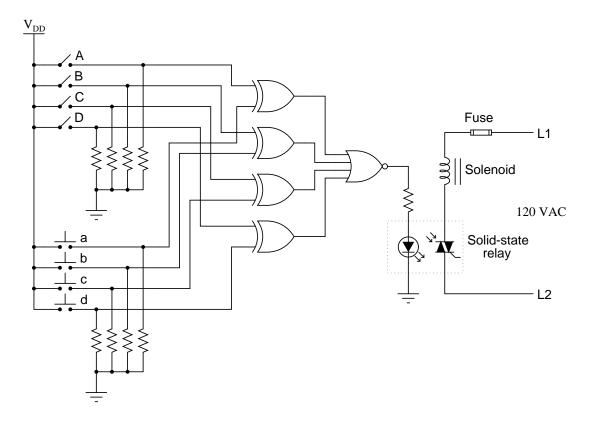
The four pushbutton switches (a, b, c, and d) are accessible to the person wishing to enter the door. The four toggle switches (A, B, C, and D) are located behind the door, and are used to set the code necessary for entering.
