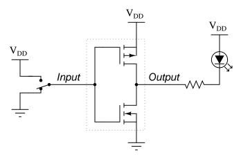
Is this gate circuit configured to source load current, sink load current, or do both?  $\underline{file}$  01259
