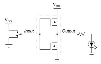
Determine the status of the LED in each of the input switch's two positions. Denote the logic level of switch and LED in the form of a truth table:
