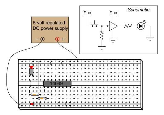
The DIP circuit is a hex inverter (it contains six "inverter" or "NOT" logic gates), but only one of these gates is being used in this circuit. The student's intent was to build a logic circuit that energized the LED when the pushbutton switch was unactuated, and de-energized the LED when the switch was pressed: so that the LED indicates the reverse state of the switch itself. The student builds this circuit, and it is found to function perfectly well.
