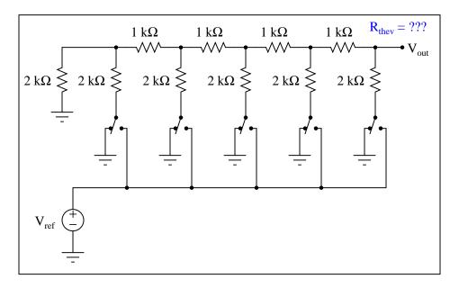
When only the most significant bit (MSB) of an R-2R ladder resistor network is activated (all other bits inactive, their switches connecting to ground), the output voltage will be the same, regardless of how many bits the network has:
