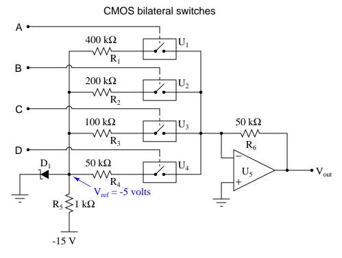
This digital-to-analog converter (DAC) circuit takes a four-bit binary input (input terminals A through D) and converts it to an analog voltage  $(V_{out})$ . Predict how the operation of this circuit will be affected as a result of the following faults. Consider each fault independently (i.e. one at a time, no multiple faults):
