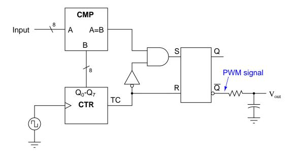
Explain how this circuit works, using timing diagrams if necessary to help show the PWM signal at  $\overline{Q}$  for different input values.
