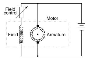
What effect will this change in field excitation do to the operating speed of the motor?  $\underline{\text{file }00551}$
