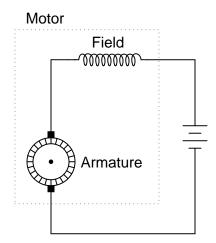
Contrast this behavior against that of a permanent magnet DC motor under the same conditions (increased mechanical load, causing counter-EMF to decrease).
