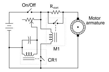
The relay labeled "M1" is a large "contactor" designed to shunt the motor's current around the start-up resistor. It requires at least a few amps of current through its coil to energize.
