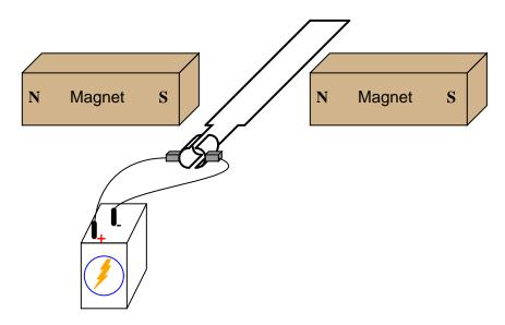
A DC motor may be thought of as a series of electromagnets, radially spaced around a common shaft:
