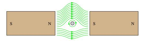
This interaction of magnetic flux lines (the bar magnets' straight lines versus the wire's circles) will produce a mechanical force on the wire (called the *Lorentz* force). Which direction will this force act? Also, determine the direction of current through the conductor (seen from an end-view in the above illustration) necessary to produce the circular magnetic flux shown.
