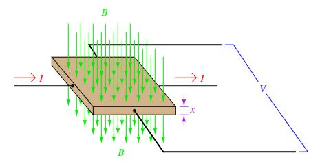
Explain what this equation means with regard to the effect of each variable (I, B, and x) on the Hall voltage generated. Identify whether each of the variables has a *direct* or an *inverse* effect on the output voltage.
