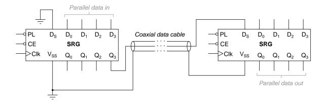
Specify what logic states would have to be input at the PL, CE, and Clk terminals of each shift register, and at what times, to successfully load four bits of parallel data, shift them serially over the coaxial data cable, and then hold them at the outputs (Q) of the receiving shift register.
