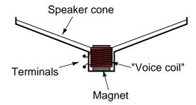
The "voice coil" is attached to the flexible speaker cone, and is free to move along the long axis of the magnet. The magnet is stationary, being solidly anchored to the metal frame of the speaker, and is centered in the middle of the voice coil.
