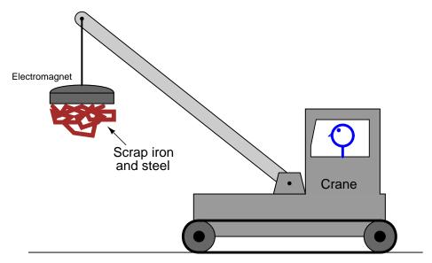
In this illustration of a crane, superimpose a drawing showing the electromagnet, electrical power supply and wiring necessary for this to work. Also include a switch so the crane operator can turn the magnet on and off. Also, draw an electrical schematic diagram of the same circuit, showing all components in the crane's magnet circuit.
