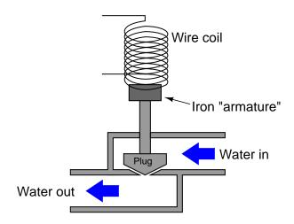
Essentially, this is an electrically-controlled on/off water valve. In the development of this valve, though, the design engineers discover that the magnetic force produced by the electromagnet coil is not strong enough to achieve reliable valve actuation every time. What can be changed in this solenoid valve design to produce a greater actuating force?
