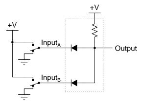
Identify what type of logic function is represented by this gate circuit (AND, OR, inverter, etc.). Also, trace the directions of all currents in this circuit.
