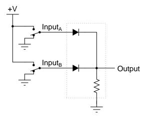
Identify what type of logic function is represented by this gate circuit (AND, OR, inverter, etc.). file 02763
