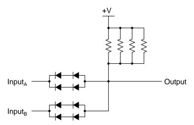
First, draw a schematic for a non-redundant, passive AND gate. Which components shown in the above schematic are "redundant," and which are essential?
