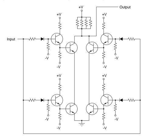
Explain why the circuit is referred to as *quad*-redundant. How many individual component failures, minimum, must occur before the gate's functionality is compromised? Prove your answer through an analysis of the circuit's operation.
