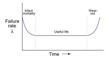
While the "Useful life" and "Wear-out" phases of the system life-cycle are easy to understand, the initial "Infant mortality" phase is not so intuitive. Explain what factors might lead to premature component failure during this initial phase of a system's lifespan.
