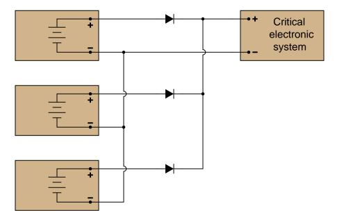
However, as an experienced electronics technician, you should know that diodes are not immune to failure. Modify this schematic diagram to include three extra (redundant) diodes that will allow normal operation if any one of the three original diodes were to fail, assuming the most common failure mode of rectifier-type diodes.
