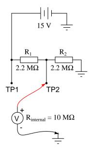
Suppose you tried to measure the voltage at all three test points with an analog voltmeter having a sensitivity rating of 20 k $\Omega$  per volt, set on the 10 volt scale. How much voltage would it indicate at each test point? How much voltage *should* it ideally indicate at each test point?
