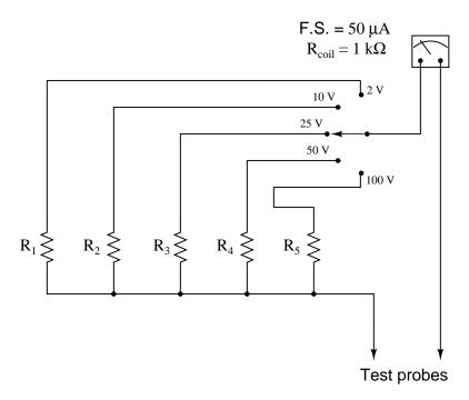
Calculate the necessary resistance values to give this multi-range voltmeter the ranges indicated by the selector switch positions:
