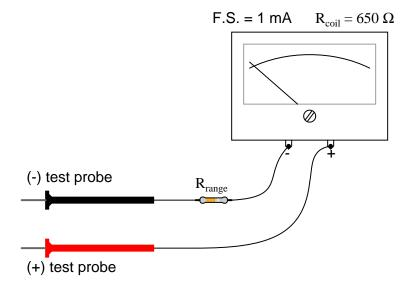
Calculate the necessary resistance value and power rating for  $R_{range}$  in order to make the meter movement respond as a voltmeter with a range of 0 to 50 volts:
