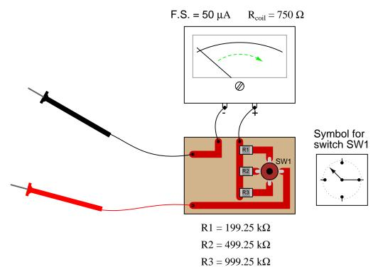
All components on the printed circuit board are "surface-mount," soldered onto the top surfaces of the copper traces. The switch (SW1) schematic diagram is shown to the immediate right of the circuit board, with resistor values shown below the circuit board.
