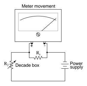
The meter movement's coil resistance  $(R_{coil})$  may be calculated following this formula:
