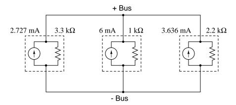
Write an algebraic equation that solves for the voltage between the two bus conductors, based on the problem-solving method of Thévenin-to-Norton conversion, combining Norton sources into one, and combining resistors into one:
