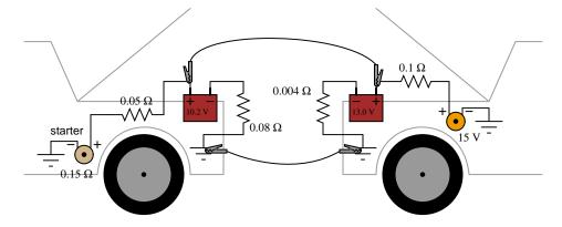
Regard the starter motor itself as a 0.15  $\Omega$  resistor, and disregard any resistance of the jumper cables connecting the two cars' electrical systems together.
