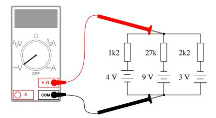
A set of batteries are connected in parallel to form a battery bank. Ideally, their individual voltages would be exactly equal, and there would be no stray resistance anywhere in the circuit, but in reality what we have is something like this:
