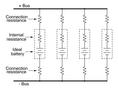
Use Millman's theorem to calculate the total voltage between the two busses for the battery bank, given these specifications for the four batteries:
