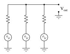
The "superposition principle" states that when two or more waveforms mix together in a linear network, the result is the sum of the waveforms. That is, the waveforms simply add up to make a total, and are not "irrevocably affected" by one another. The question, then, is really: what constitutes a *linear* network?
