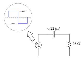
No, I'm not asking you to calculate an infinite number of terms in the Fourier series – that would be cruel and unusual. Just calculate the power dissipated in the resistor by the 1st, 3rd, 5th, and 7th harmonics only.
