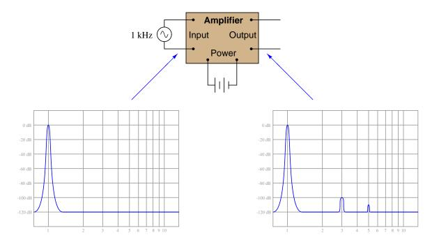
Interpret the two graphical displays and explain why the output signal has more "peaks" than the input. What is this difference telling us about the amplifier's performance?  $\frac{\text{file }03307}{\text{file }03307}$
