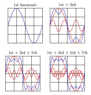
Here is what the composite wave would look like if we added all odd-numbered harmonics up to the 13th together, following the same pattern of diminishing amplitudes:
