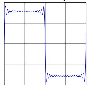
This mathematical equivalence between a square wave and the weighted sum of all odd-numbered harmonics is very useful in analyzing AC circuits where square-wave signals are present. From the perspective of AC circuit analysis based on sinusoidal waveforms, how would you describe the way an AC circuit "views" a square wave?
