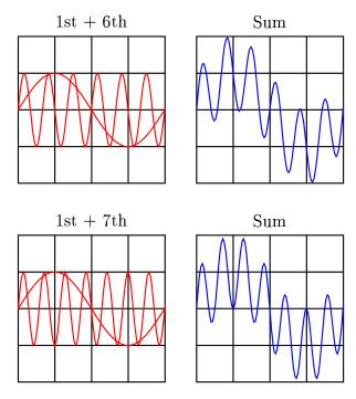
Examine these sets of harmonic sums, and indicate the trend you see with regard to harmonic number and symmetry of the final (Sum) waveforms. Specifically, how does the addition of an even harmonic compare to the addition of an odd harmonic, in terms of final waveshape?
