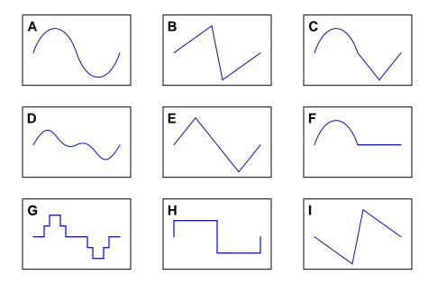
Note that only one cycle is shown for each waveform. Remember that we're dealing with continuous waveforms, endlessly repeating, and not single cycles as you see here.
