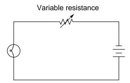
This method of electrical power control is not without its disadvantages, though. Consider an example where the circuit current is 5 amps, the variable resistance is 2  $\Omega$ , and the lamp drops 20 volts of voltage across its terminals. Calculate the power dissipated by the lamp, the power dissipated by the variable resistance, and the total power provided by the voltage source. Then, explain why this method of power control is not ideal.
