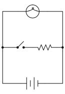
What would happen if a wire having no resistance at all  $(0 \Omega)$  were connected directly across the terminals of a 6-volt battery? How much current would result, according to Ohm's Law?
