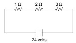
In this circuit, three resistors receive the same amount of voltage (24 volts) from a single source. Calculate the amount of current "drawn" by each resistor, as well as the amount of power dissipated by each resistor:
