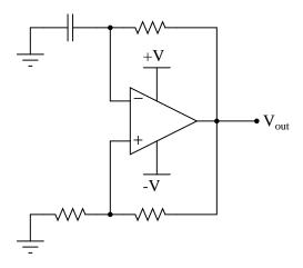
Dual, or split, power supplies are very useful in opamp circuits because they allow the output voltage to rise above as well as sink below ground potential, for true AC operation. In some applications, though, it may not be practical or affordable to have a dual power supply to power your opamp circuit. In this event, you need to be able to figure out how to adapt your dual-supply circuit to single-supply operation.
