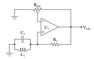
The reason for this choice in potentiometers is to make accidental changes in circuit gain less probable. If you build this circuit, you will see that tiny changes in this potentiometer's setting make a huge difference in the quality of the output sine wave. A little too much gain, and the sine wave becomes noticeably distorted. Too little gain, and the circuit stops oscillating altogether!
