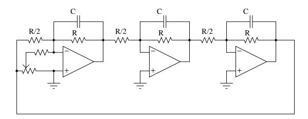
With all the resistors and capacitors, you might have guessed this to be a phase-shift type of oscillator circuit, and you would be correct. Here, each parallel RC network provides 60 degrees of lagging phase shift to combine with the 180 degrees of phase shift inherent to the inverting amplifier configurations, yielding 120 degrees of shift per opamp stage.
