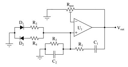
With this network in place, the circuit gain may be adjusted well above the threshold for oscillation (Barkhausen criterion) without exhibiting excessive distortion as it would have without the limiting network. Explain why the limiting network makes this possible.
