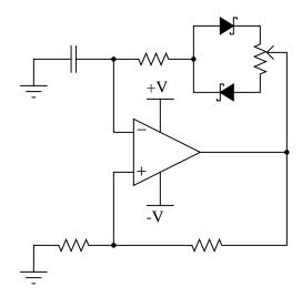
Explain how this circuit works, and which direction the potentiometer wiper must be moved to increase the duty cycle (more time spent with the opamp output saturated at +V and less time spent saturated at -V).
