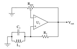
This resonant LC oscillator circuit is very sensitive to changes in the gain. Note how the potentiometer used in this circuit is the "trimmer" variety, adjustable with a screwdriver rather than by a knob or other hand control:
