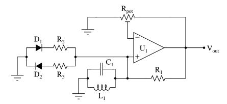
With this network in place, the circuit gain may be adjusted well above the threshold for oscillation (Barkhausen criterion) without exhibiting excessive distortion as it would have without the limiting network. Explain why the limiting network makes this possible.
