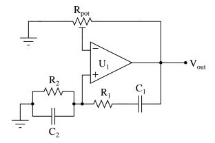
The reason for this choice in potentiometers is to make accidental changes in circuit gain less probable. If you build this circuit, you will see that tiny changes in this potentiometer's setting make a huge difference in the quality of the output sine wave. A little too much gain, and the sine wave becomes noticeably distorted. Too little gain, and the circuit stops oscillating altogether!
