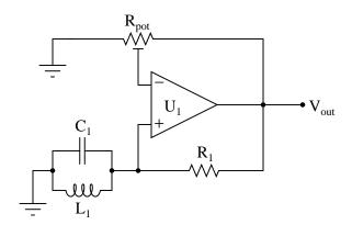
How many degrees of phase shift must the feedback circuit (the square box in this schematic) introduce to the signal in order for this inverting amplifier circuit to oscillate?
