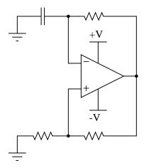
First, determine what would happen if we were to simply eliminate the negative portion of the dual power supply and try to run the circuit on a single supply (+V and Ground only):
