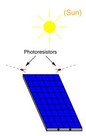
Two comparators are used to sense the differential resistance produced by these two LDR's, and activate a tracking motor to tilt the solar panel on its axis when the differential resistance becomes too great. An "H-drive" transistor switching circuit takes the comparators' output signals and amplifies them to drive a permanent-magnet DC motor one way or the other:
