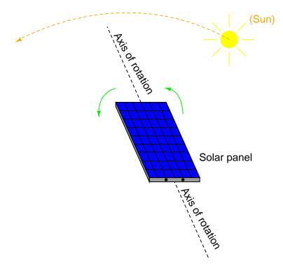
One way to detect the sun's position relative to the panel is to attach a pair of Light-Dependent Resistors (LDR's) to the solar panel in such a way that each LDR will receive an equal amount of light only if the panel is pointed directly at the sun:
