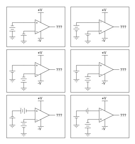
Determine the output voltage polarity of this op-amp (with reference to ground), given the following input conditions:
