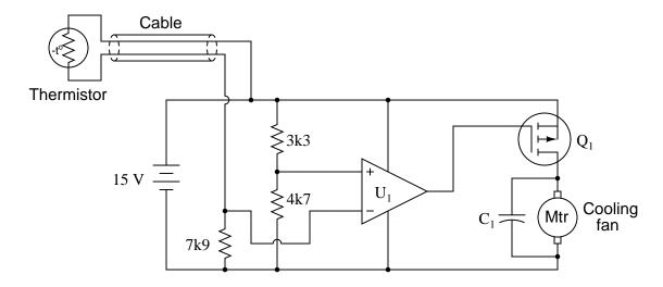
Predict how the operation of this thermostat circuit (where the cooling fan motor is supposed to turn on when the temperature gets too high) will be affected as a result of the following faults. Consider each fault independently (i.e. one at a time, no multiple faults):
