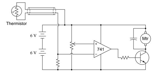
The circuit works just as it is supposed to in turning the motor on and off, but it has a strange problem: the transistor gets warm when the motor is *off!* Oddly enough, the transistor actually cools down when the motor turns on.
