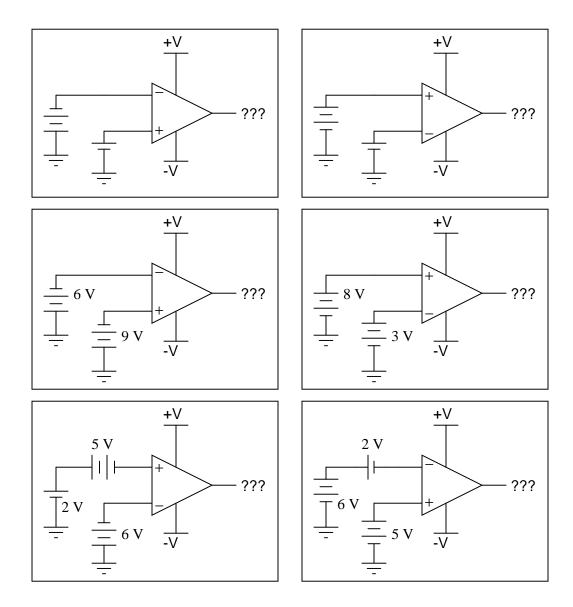
Although the following symbol is generally interpreted as an operational amplifier ("op-amp"), it may also be used to represent a comparator:
