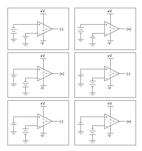
In these illustrations, I have likened the op-amp's action to that of a single-pole, double-throw switch, showing the "connection" made between power supply terminals and the output terminal.
