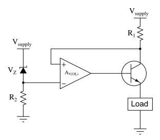
Explain how this op-amp really does provide negative feedback, which of course is necessary for stable current regulation, as positive feedback would be completely unstable.  $\underline{file~03942}$
