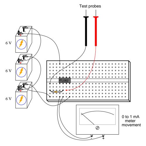
Draw a schematic diagram of this circuit, a calculate the resistor value necessary to give the meter a voltage measurement range of 0 to 5 volts.
