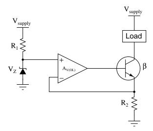
Write an equation solving for the regulated load current, given any relevant variables shown in the schematic diagram  $(R_1, V_Z, V_{supply}, A_{V(OL)}, \text{ etc.})$ .
