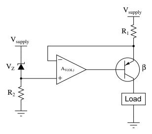
Write an equation solving for the regulated load current, given any relevant variables shown in the schematic diagram  $(R_1, V_Z, V_{supply}, A_{V(OL)}, \text{ etc.})$ . Also, describe what would have to be changed in this circuit in order to set the regulated current at a different value.
