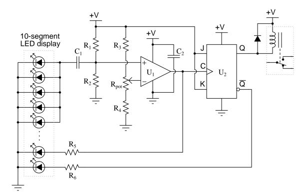
Of course, you are not restricted to using this exact design. One variation is to place a monostable 555 timer circuit at the output of the comparator instead of a J-K flip-flop. This would activate the output for a certain time period after detecting a pulse of light, rather than using one light pulse to turn the output on and another light pulse to turn the output off.
