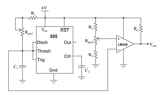
$R_1$ ,  $R_{pot1}$ , and  $C_1$  set the oscillation frequency.  $R_{pot2}$  sets the duty cycle.
