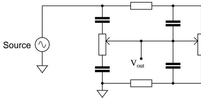
Determine which potentiometer controls the bass (low frequency) tones and which controls the treble (high frequency) tones, and explain how you made those determinations.
