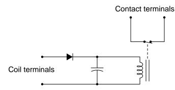
Explain how this circuit works, and also determine what type of time-delay relay function is provided by it (NOTO, NOTC, NCTO, or NCTC). <u>file 03140</u>
