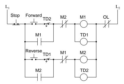
What extra functionality do the time-delay relays contribute to this motor control circuit? <u>file 03148</u>
