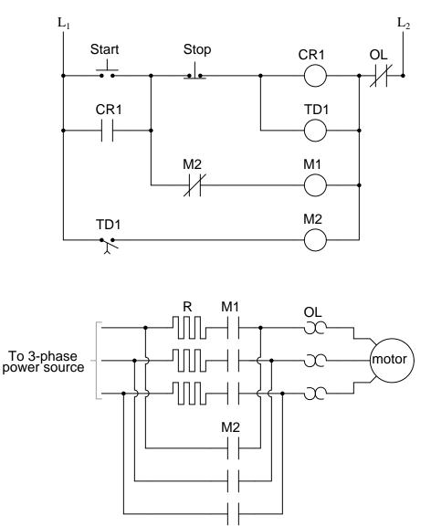
Analyze this ladder logic diagram, and explain how it starts up the electric motor more gently than an "across-the-line" starter would.
