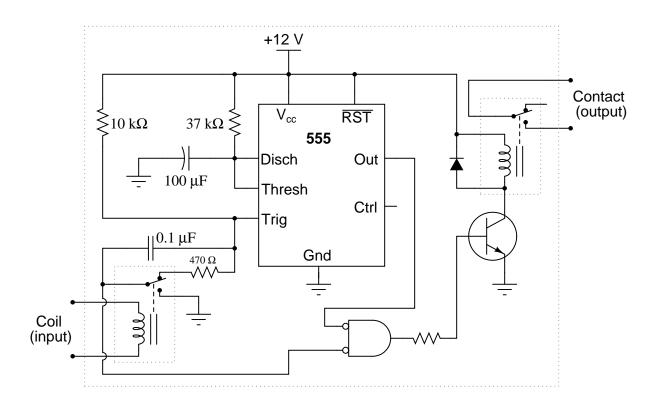
Also, calculate the amount of delay, in seconds. Hint: the 555's timing capacitor will charge from 0 volts to  $\frac{2}{3}$  supply voltage during the charging cycle.
