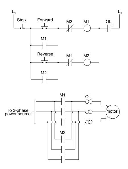
Study this diagram, then explain how motor reversal is accomplished. Also, identify the function of each "M" contact in the control circuit, especially those normally-closed contacts in series with the motor starter coils.
