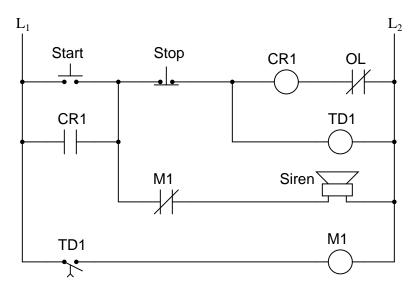
However, this circuit is poorly designed. Although it works just fine under normal conditions, it may not do what it should in the event of an overload heater trip (if the normally-closed "OL" contact opens). Explain what is wrong with this circuit.
