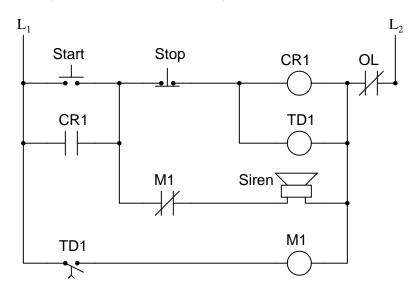
Unfortunately, there is a problem somewhere in this circuit. Instead of activating the siren before starting the motor, there is silence. The motor's start is still delayed by the correct amount of time, but the siren never makes a sound. Identify some possible causes of this problem. Also, identify portions of the circuit you know to be functioning properly.
