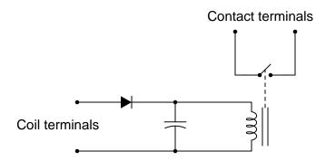
Explain how this circuit works, and also determine what type of time-delay relay function is provided by it (NOTO, NOTC, NCTO, or NCTC). <u>file 03139</u>
