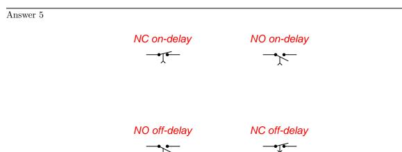
Follow-up question: how do you make sense of the arrow in each contact symbol, with regard to whether the contact is an "on-delay" or an "off-delay"?
