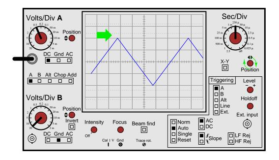
Now, the point at which the waveform triggers is clearly visible, no longer hidden from view past the left-hand side of the screen:
