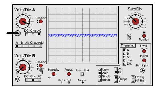
Explain what setting(s) the student can change on the oscilloscope to properly trigger this waveform so it will "hold still" on the screen.
