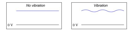
The vibration sensing circuitry measures the amplitude of this ripple and initiates a shutdown if it exceeds a pre-determined value.
