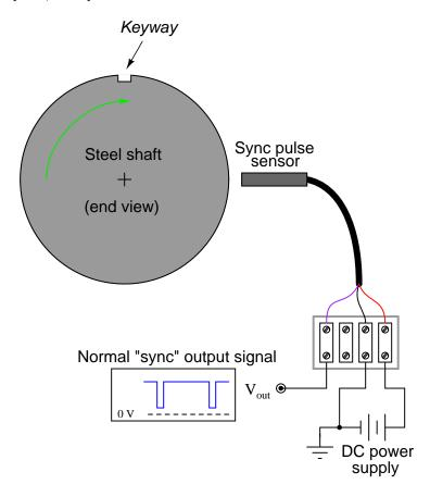
The purpose of this "sync" pulse is to provide an angular reference point, so any vibration peaks seen on any of the other sensor signals may be located relative to the sync pulse. This allows a technician or engineer to determine where in the shaft's rotation any peaks are originating.
