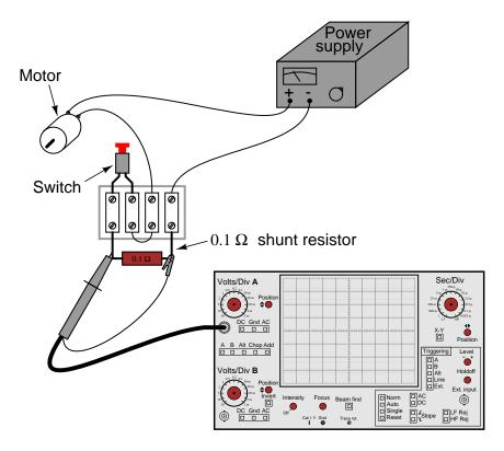
Explain how this circuit configuration enables the oscilloscope to measure motor current, when it plainly is a voltage-measuring instrument.
