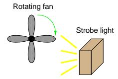
One problem with using a strobe light is that the frequency of the light pulses must exactly match the frequency of the object's rotation, or else the object will not appear to stand still. If the flash rate is mismatched, even by the slightest amount, the object will appear to *slowly* rotate instead of stand still.
