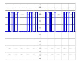
This is a difficult waveform to trigger, because there are so many identical leading and trailing edges to trigger from. No matter where the trigger level control is set, or whether it is set for rising- or falling-edge, the waveform will tend to "jitter" back and forth horizontally on the screen because these controls cannot discriminate the *first* pulse from the other pulses in each cluster of pulses. At the start of each "sweep," *any* of these pulses are adequate to initiate triggering.
