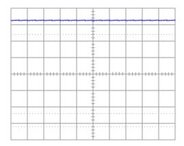
After switching the input channel's coupling control to "AC", the student increases the vertical sensitivity (fewer volts per division) to magnify the ripple voltage. The problem is, the ripple waveform is not engaging the oscilloscope's triggering. Instead, all the student sees is a blur as the waveform quickly scrolls horizontally on the screen:
