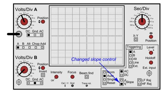
Draw the waveform's new appearance on the oscilloscope screen, with the slope control reversed.  $\underline{\text{file }01908}$
