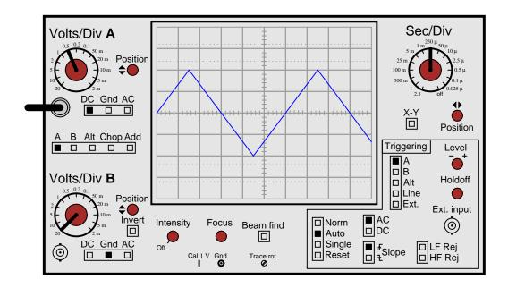
The horizontal position knob is then turned clockwise until the left-hand edge of the waveform is visible:
