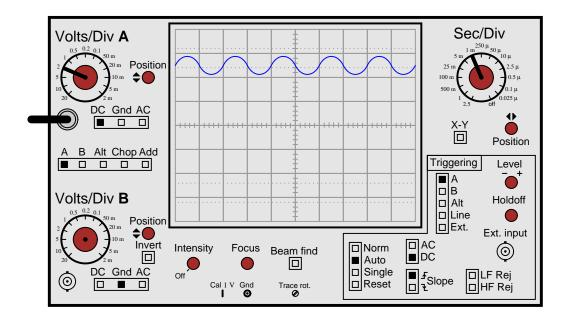
A student wants to measure the "ripple" voltage from an AC-DC power supply. This is the small AC voltage superimposed on the DC output of the power supply, that is a natural consequence of AC-to-DC conversion. In a well-designed power supply, this "ripple" voltage is minimal, usually in the range of millivolts peak-to-peak even if the DC voltage is 20 volts or more. Displaying this "ripple" voltage on an oscilloscope can be quite a challenge to the new student.
