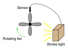
The only way to consistently guarantee a repetitive waveform will appear "still" on an analog oscilloscope screen is for each left-to-right sweep of the CRT's electron beam to begin at the same point on the waveform. Explain how the "trigger" system on an oscilloscope works to accomplish this. file 01905
