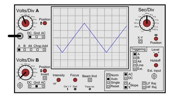
This student's oscilloscope is set on the *Norm* mode. If it were set on the *Auto* mode, the trace would default to "free-running" if ever the trigger level were set above or below the waveform's amplitude. Instead of completely disappearing, the waveform would scroll horizontally and not "stand still" if the trigger level were set too high or too low.
