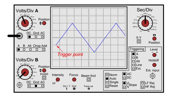
What will happen now if the trigger level knob is turned clockwise? How will this affect the positioning of the waveform on the oscilloscope screen?
