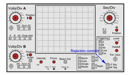
Follow-up question: identify the filter circuits internal to the oscilloscope associated with each of these "rejection" controls.
