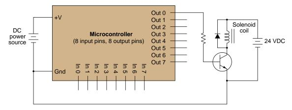
Unfortunately, a single BJT does not provide enough current gain to actuate the solenoid. With 20 mA of output current from the microcontroller pin and a  $\beta$  of only 25 (typical for a power transistor), this only provides about 500 mA to the solenoid coil.
