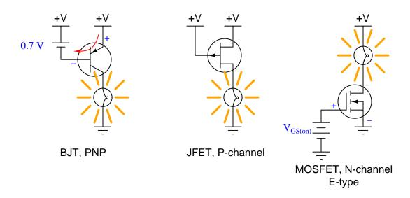
Follow-up question: for the JFET, which is already "on" with zero voltage applied to the gate, describe what would be necessary to force it into the "off" state.
