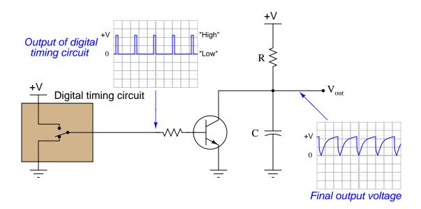
First, identify what signal level from the digital circuit ("high" or "low") causes the capacitor to charge, and what level causes it to discharge. Then, replace the BJT with a suitable MOSFET to accomplish the exact same timing function:
