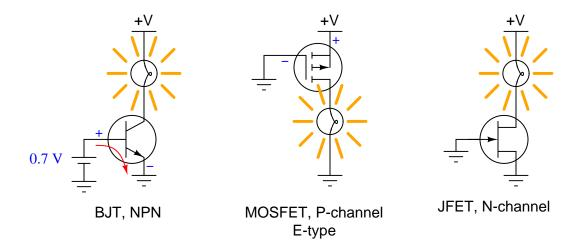
Follow-up question: for the JFET, which is already "on" with zero voltage applied to the gate, describe what would be necessary to force it into the "off" state.
