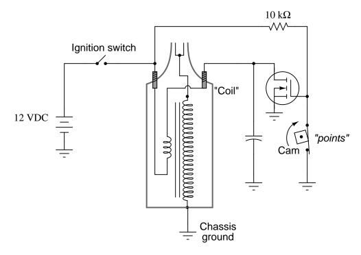
Explain how this revised circuit works. When does the MOSFET conduct current, when the point
