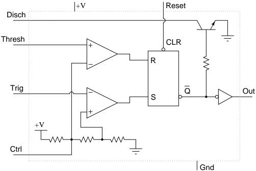
The various inputs and outputs of this circuit are labeled in the above schematic as they often appear in datasheets ("Thresh" for *threshold*, "Ctrl" or "Cont" for *control*, etc.).
