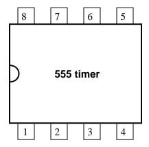
The model "555" integrated circuit is a very popular and useful "chip" used for timing purposes in electronic circuits. The basis for this circuit's timing function is a resistor-capacitor (RC) network:
