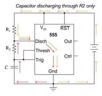
Note that this second current (through the battery) does not go anywhere near the capacitor, and so is irrelevant to the discharge cycle time.
