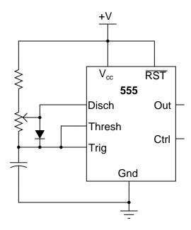
With the diode in place, the output waveform's duty cycle may be adjusted to less than 50% if desired. Explain why the diode is necessary for that capability. Also, identify which way the potentiometer wiper must be moved to decrease the duty cycle.
