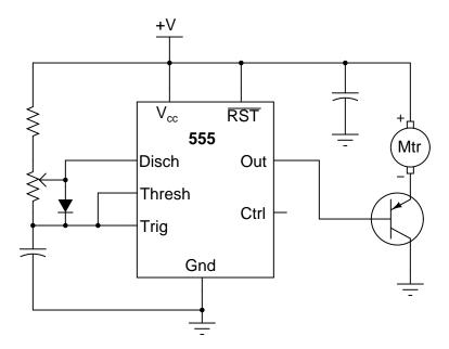
One of the major advantages to using PWM to proportion power to a load is that the final switching transistor operates with minimal heat dissipation. If we were to use a transistor in its linear ("active") mode, it would dissipate far more heat when controlling the speed of this motor! By dissipating less heat, the circuit wastes less power.
