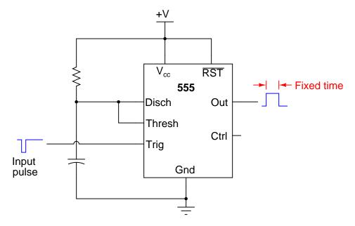
How low does the triggering voltage have to go in order to initiate the output pulse? Also, write an equation specifying the width of this pulse, in seconds, given values of R and C. Hint: the magnitude of the supply voltage is irrelevant, so long as it does not vary during the capacitor's charging cycle. Show your work in obtaining the equation, based on equations of RC time constants. Don't just copy the equation from a book or datasheet!
