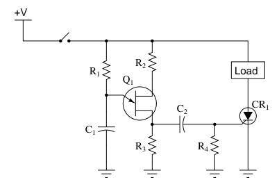
Together, the combination of  $R_1$ ,  $C_1$ ,  $R_2$ ,  $R_3$ , and  $Q_1$  form a relaxation oscillator, which outputs a square wave signal. Explain how a square wave oscillation is able to perform a simple time-delay for the load, where the load energizes a certain time after the toggle switch is closed. Also explain the purpose of the RC network formed by  $C_2$  and  $R_4$ .
