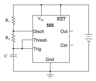
Base your equations on the general rules of RC time constant circuits. Don't just copy the completed equations from some reference book! Assume that the 555's discharge transistor is a perfect switch when turned on (0 volts drop). Note that the supply voltage is irrelevant to these calculations, so long as it remains constant during the charging cycle.
