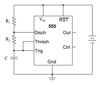
In this configuration, the "555" chip acts as an *oscillator*: switching back and forth between "high" (full voltage) and "low" (no voltage) output states. The time duration of one of these states is set by the charging action of the capacitor, through both resistors ( $R_1$  and  $R_2$  in series). The other state's time duration is set by the capacitor discharging through one resistor ( $R_2$ ):
