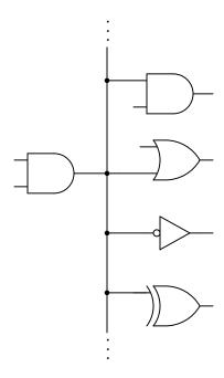
Explain why this limit exists. What is it about the construction of TTL logic gates that inherently limits the number of TTL inputs that any one TTL output can drive? What might happen if this limit is exceeded?
