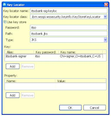
Figure 9-72 Key locator for message signing key
