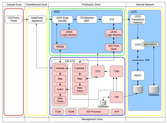
Figure 8-14 Complete solution design
