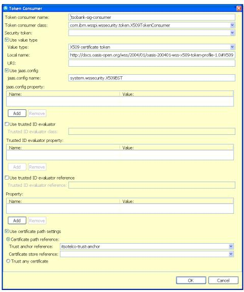
Figure 9-13 Token consumer for certificate used to validate the message certificate
