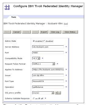
Figure 9-45 Federated Identity Manager configuration settings
