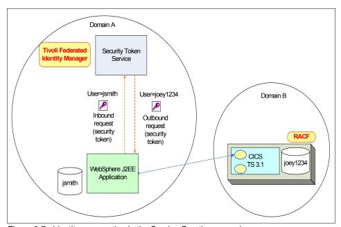
Figure 3-7 Identity propagation in the Service Creation scenario
