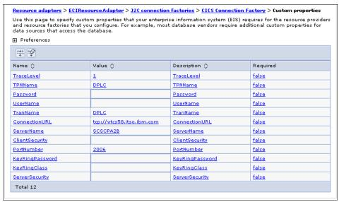
Figure 9-82 Custom properties for CICS connection factory
