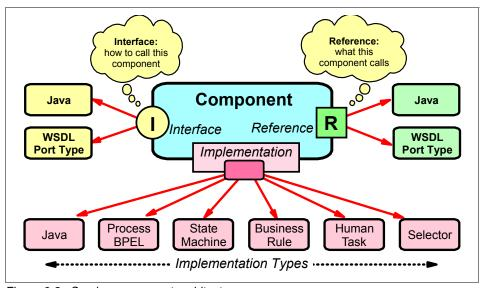
Figure 6-3 Service component architecture
