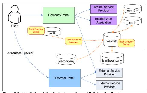
Figure 5-5 Identity foundation for the Interaction and Collaboration Services scenario
