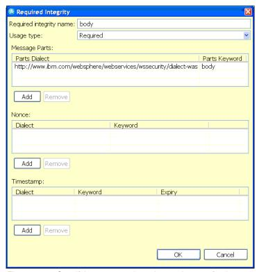
Figure 9-11 Specifying message integrity requirement for the response body
