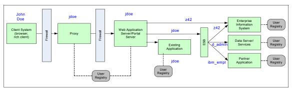
Figure 2-6 Identity provisioning example
