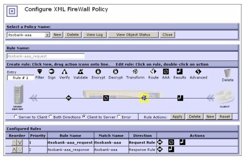
Figure 9-52 Adding a transform action
