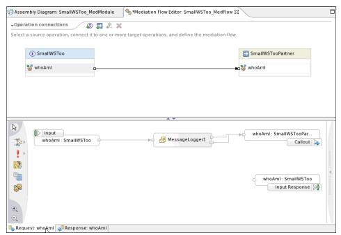
Figure 12-3 Simple mediation flow with MessageLogger only
