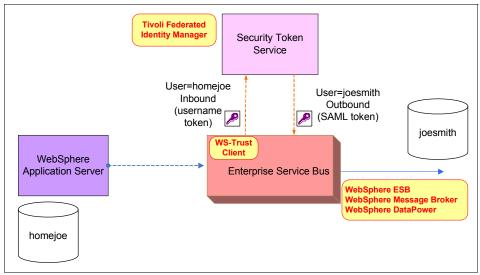
Figure 4-2 Identity propagation at the ESB
