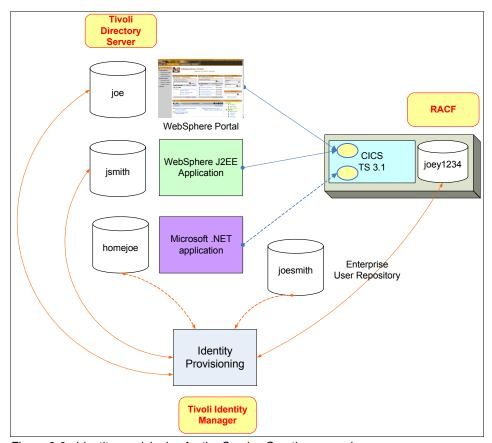
Figure 3-6 Identity provisioning for the Service Creation scenario
