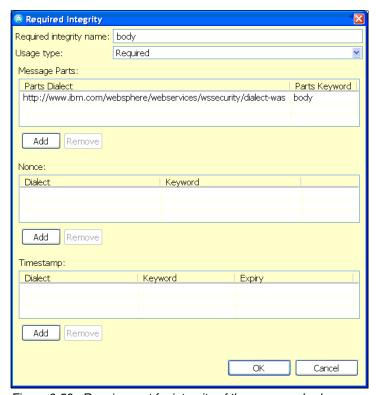
Figure 9-59 Requirement for integrity of the message body
