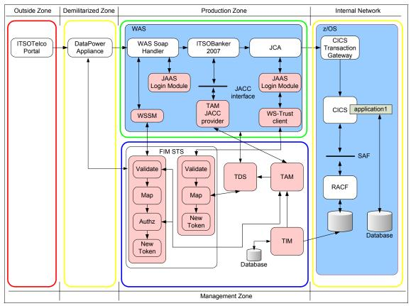
Figure 8-11 Components - JACC Provider
