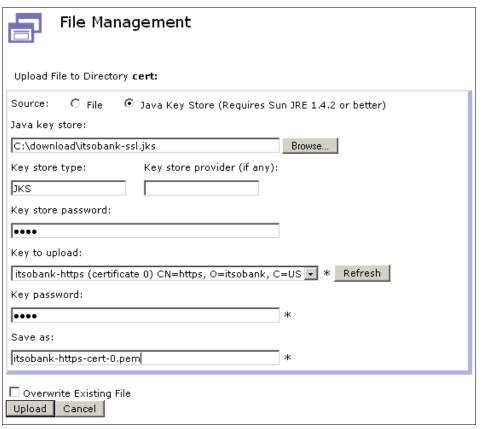
Figure 9-35 Selecting the certificate for the SSL listener
