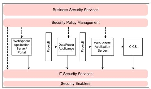
Figure 8-2 Applying the IBM SOA Security Reference Model
