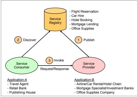
Figure A-2 SOA components and operations
