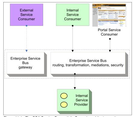
Figure 11-1 The SOA Service Connectivity Scenario architecture pattern
