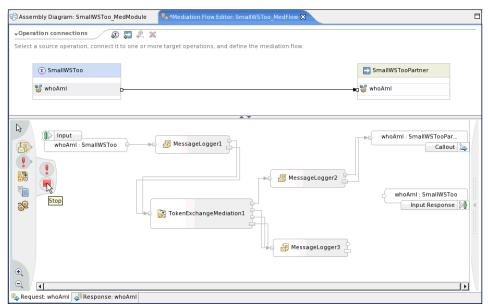
Figure 12-6 Mediation Flow with the TokenExchangeMediation primitive
