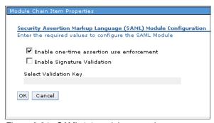
Figure 9-94 SAML 1.1 module properties
