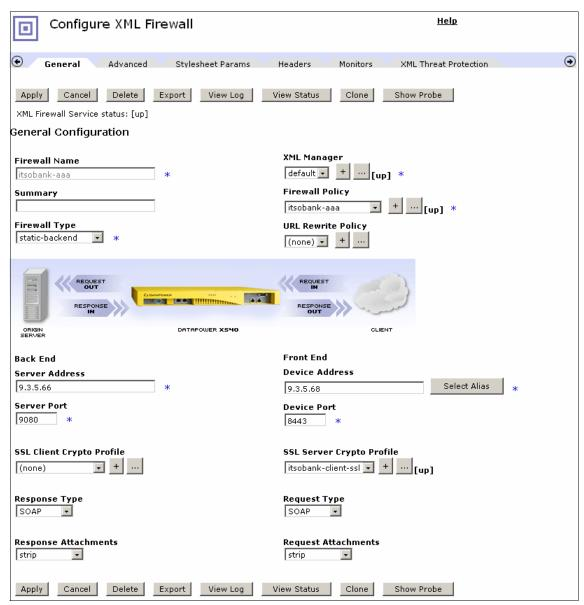
Figure 9-50 XML Firewall configuration window
