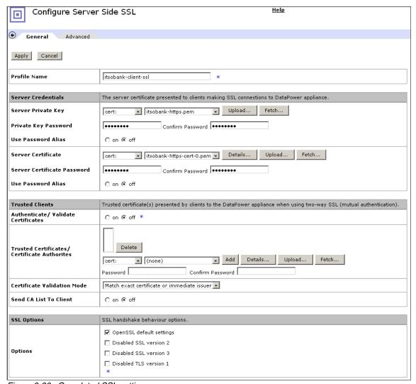
Figure 9-36 Completed SSL settings
