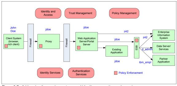
Figure 2-7 Addressing the requirements around identity propagation and mapping
