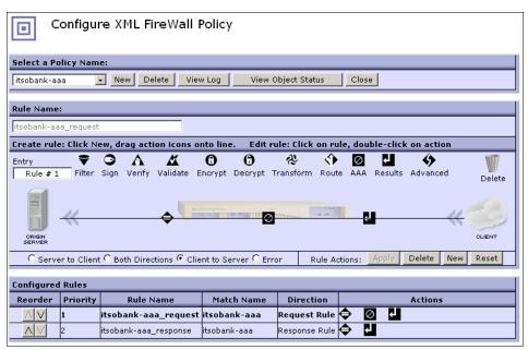
Figure 9-51 Firewall policy configuration window
