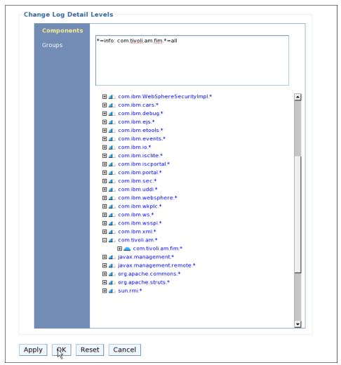
Figure 12-37 Enable Federated Identity Manager trace
