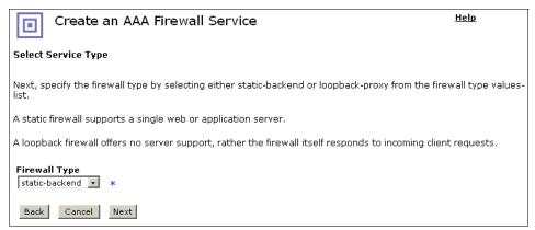
Figure 9-29 Selecting the firewall service type
