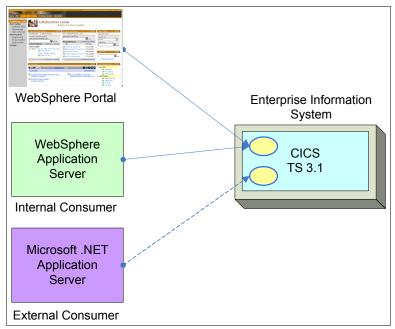
Figure 3-1 Directly exposing existing applications as services
