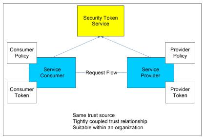
Figure 2-16 Tightly coupled trust relationship
