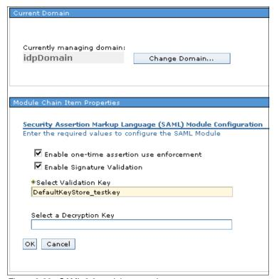
Figure 9-89 SAML 2.0 module properties
