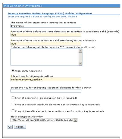
Figure 9-25 SAML 2.0 module properties
