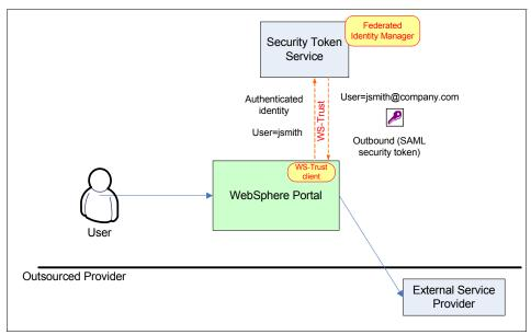
Figure 5-8 Identity propagation for the Interaction and Collaboration Services scenario: Access to an external Web service
