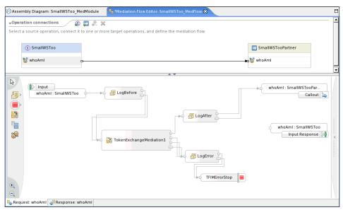
Figure 12-8 Mediation flow with renamed primitives
