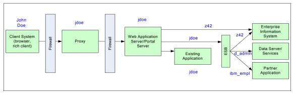
Figure 2-5 Identity propagation and mapping example
