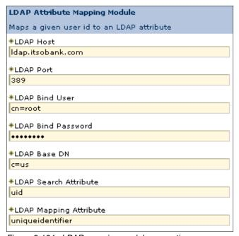
Figure 9-104 LDAP mapping module properties
