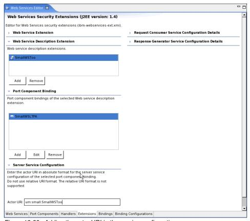
Figure 12-20 Adding the actor URI in the service configuration
