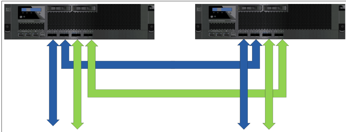
Figure 6-6 The second set of paired ports forwarding mirrored traffic over the links to the partner appliance
