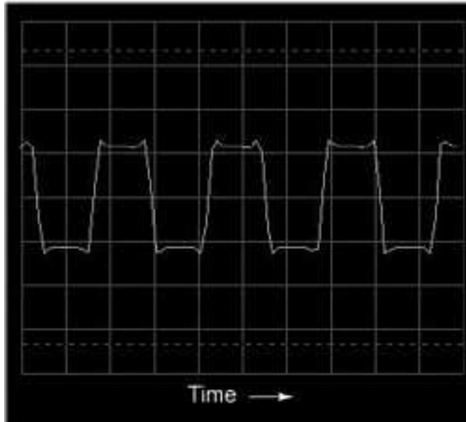
Figure 7.31: Oscilloscope time-domain display of a square wave
