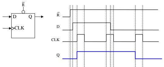
It's important to note that ^R going low before the first clock pulse forces Q to 0.
