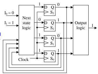
The current state is the value stored in the latches and found at the Q outputs. In the case of the diagram above, that is 0-1-0-1 with  $S_3$  being the most significant bit.
