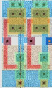
(4) Expose resist using n-well mask
