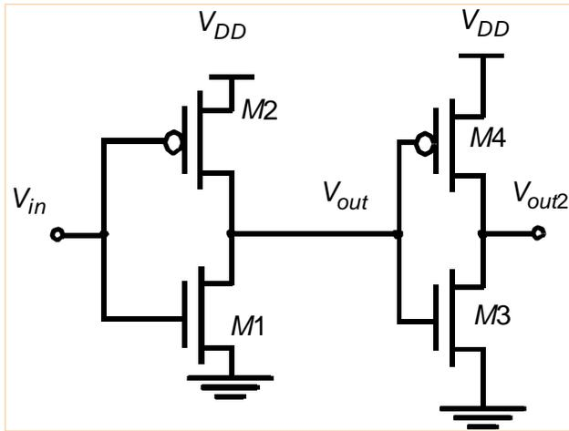
This two-inverter circuit (of Figure 3.25 in Rabaey's text ) will be manufactured in a twin-well process.
