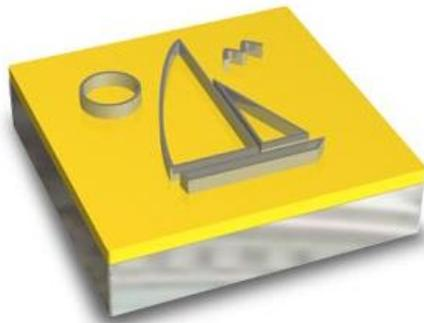
The hardened photoresist is then removed by washing with acid and the seascape is finished. We can now photograph it through a microscope and add it to the gallery in the Silicon Zoo.
