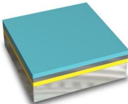
A thin film of photoresist (blue layer) is applied to the surface of the entire wafer, which is then spun at high speed to evenly spread the viscous fluid-like photoresist across the surface.
