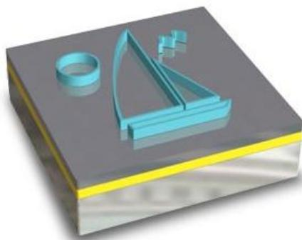
The soft unexposed photoresist is removed with an organic solvent leaving only those areas that were hardened by exposure to the ultraviolet light. An outline of the seascape is now in place.
