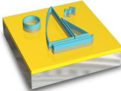
The exposed areas of aluminum metal are now removed by "etching" the surface of the wafer in a process called ion beam milling that removes the unprotected aluminum.
