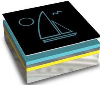
A mask containing the pattern of the sailboat, the sun, and a seagull is then placed over the wafer and ultraviolet light is then passed through the pattern exposing the soft photoresist beneath.
