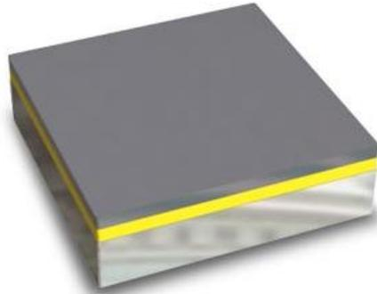
Next, a thin layer of aluminum (gray layer) is applied by vacuum metallization directly on top of the silicon dioxide layer. This material will ultimately become the "silicon seascape".
